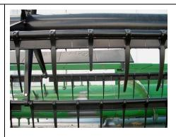
2. Slide the Quick Finger over the broken tine until it snaps in place over the rounded edge at the base of the original tine.
