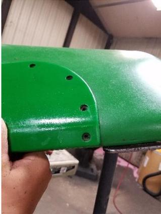
4. With the hardware provided install the self tapping screws in each of the predrilled holes on the wear panel.
