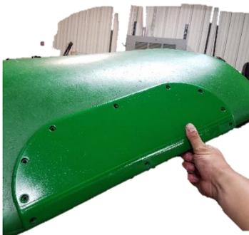
3. It is recommended to place the wear panel near the center of the snout making sure the bottom of the wear panel and the bottom of the snout is in line as shown.
